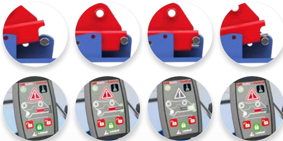
Quickcoupler unlocked, not yet fully in adapter
